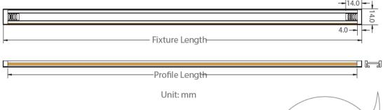
Standard Power Track lengths 1000mm / 1500mm / 2500mm (can be cut down to any length, additional end caps can be supplied) Available in White and Black color
